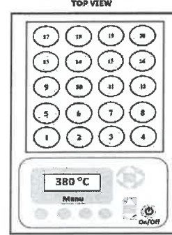
Figure 1. Location of Reference Standard and Block Diagram of Digestion Unit
